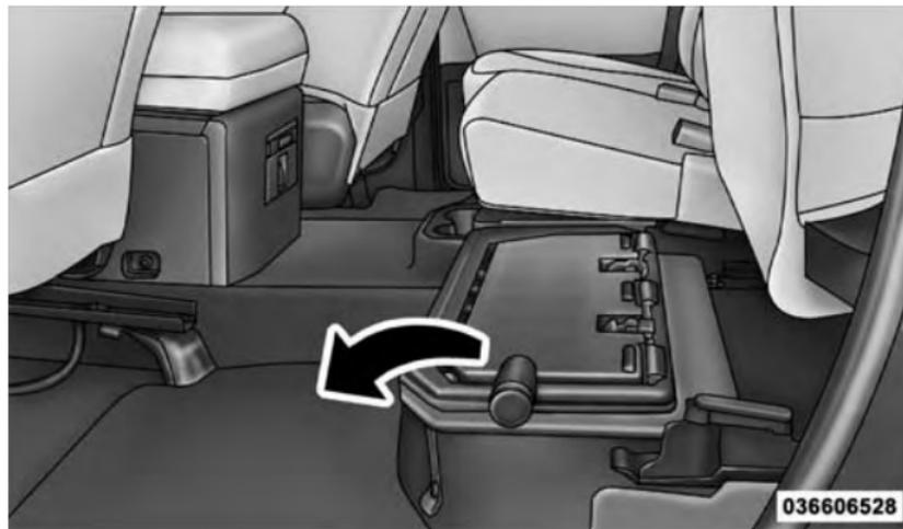
Unfolding The Load Floor
