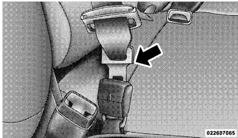
Inserting Latch Plate
