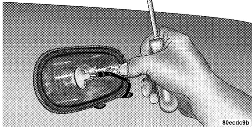
3. Pull the bulb straight from its socket and replace.
